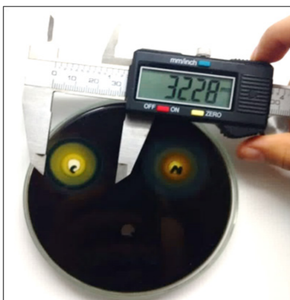
Fig.1 - Measurement of inhibition halos with a calibrated digital vernier.
